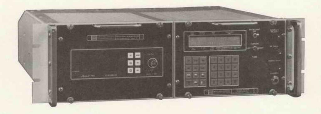
The SYS007 Signal Strength Measurement System was designed to collect signal strength versus latitude and longitude information in the 825 to 845 MHz and 870 to 890 MHz frequency ranges. It has an IF bandwidth of 20 kHz and can measure signal strength from -110 to -20 dBm.
